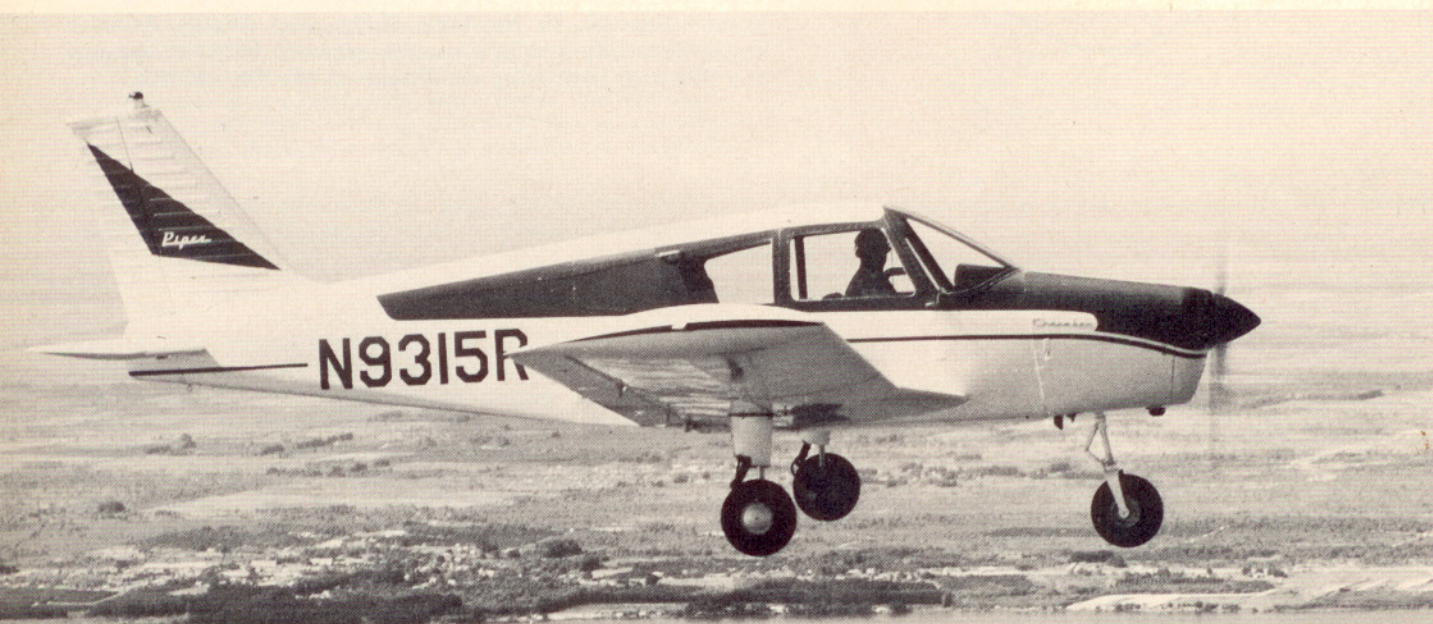
A complete departure from old designs, the Cherokee is gaining a reputation for its superb ground-handling characteristics. Note the new model's wide, tricycle gear in the photograph. It is now in production at Piper Aircraft's Vero Beach, Fla., factory
